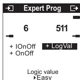
NB: the + symbol located before the **LogVal** object indicates that a group address is associated with the object.
